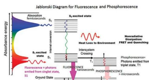
Fig. 3: The Jablonski Diagram of molecular absorbance and fluorescence
