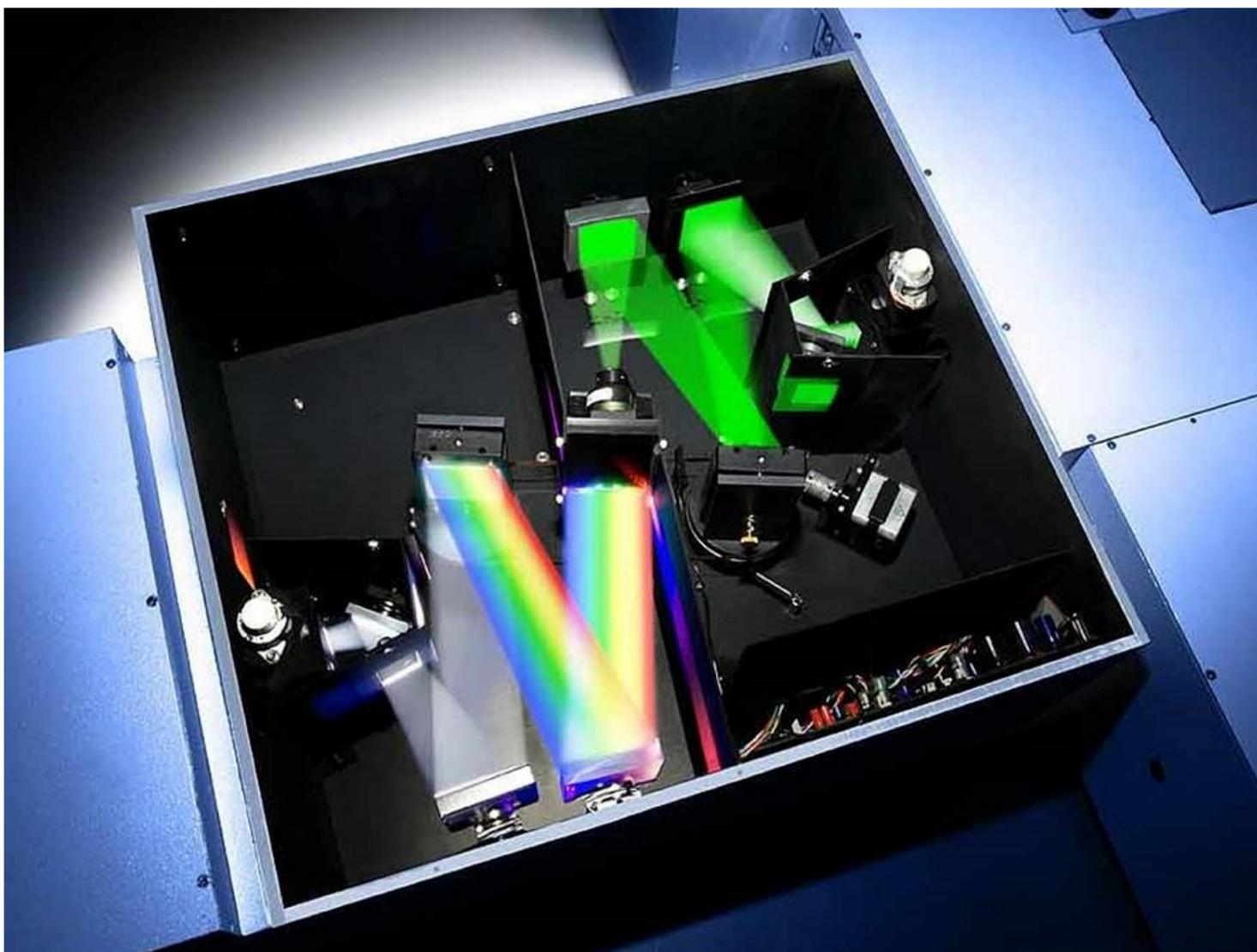
HORIBA Scientific Double Monochromator used for stray light rejection
