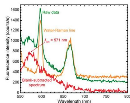
Fig. 9: Blank-subtracted emission spectrum (red) of red microspheres at  $6.7 \times 10^4$  beads/mL (exc=542 nm): The non-subtracted spectrum is green. Here, two water Raman peaks for -OH bending and stretching modes (corresponding to 3380 and 1700  $\text{cm}^{-1}$ ) can be shown in the spectrum of the blank solvent (orange) and subtracted from the sample
