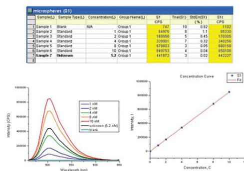
Fig. 7: Top: Table of single point intensities for a calibration curve of fluorescent microspheres in different concentrations in solution measured on a FluoroMax-4 spectrofluorometer. Bottom Left: Spectra for the same microspheres. Bottom Right: Intensity vs. Concentration with a linear fit to the calibration curve.
