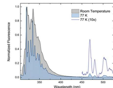
Fig. 8: Temperature can add thermal broadening to fluorescence spectra and increase phosphorescence quenching. Spectra of naphthalene dissolved in methanol measured at room temperature (298K) and in a liquid nitrogen dewar accessory (77K) on a HORIBA Fluorolog-3. The low temperature spectrum reveals rich vibrational structure and longer wavelength phosphorescence. Phosphorescence peaks are also shown magnified 10x for clarity. (HORIBA FluoroMax Series, n.d.)
