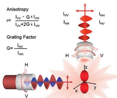
Fig. 12: Depiction of fluorescence anisotropy experiment using excitation and emission polarizers rotated to 0 degrees (Vertical, V) and 90 degrees (Horizontal, H) orientations.
