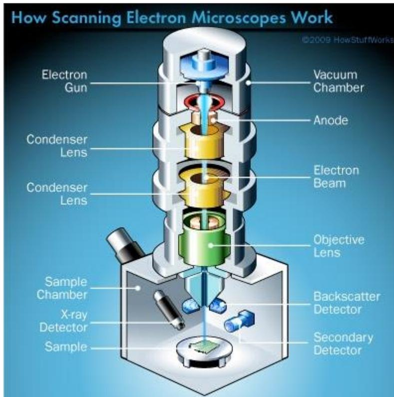
**5 Principle:** When the accelerated primary electrons strike the sample, it produces secondary electrons. These secondary electrons are collected by a positive charged electron detector which in turn gives a 3-dimensional image of the sample.
