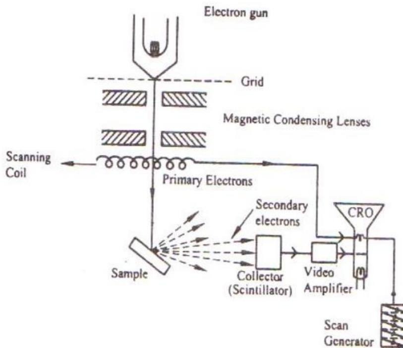
These signals can be fed into CRO through video amplifier as shown. Therefore, Scanning electron microscope consists two main parts,
